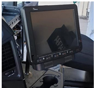
FM10Q VMC installed firmly on the truck
